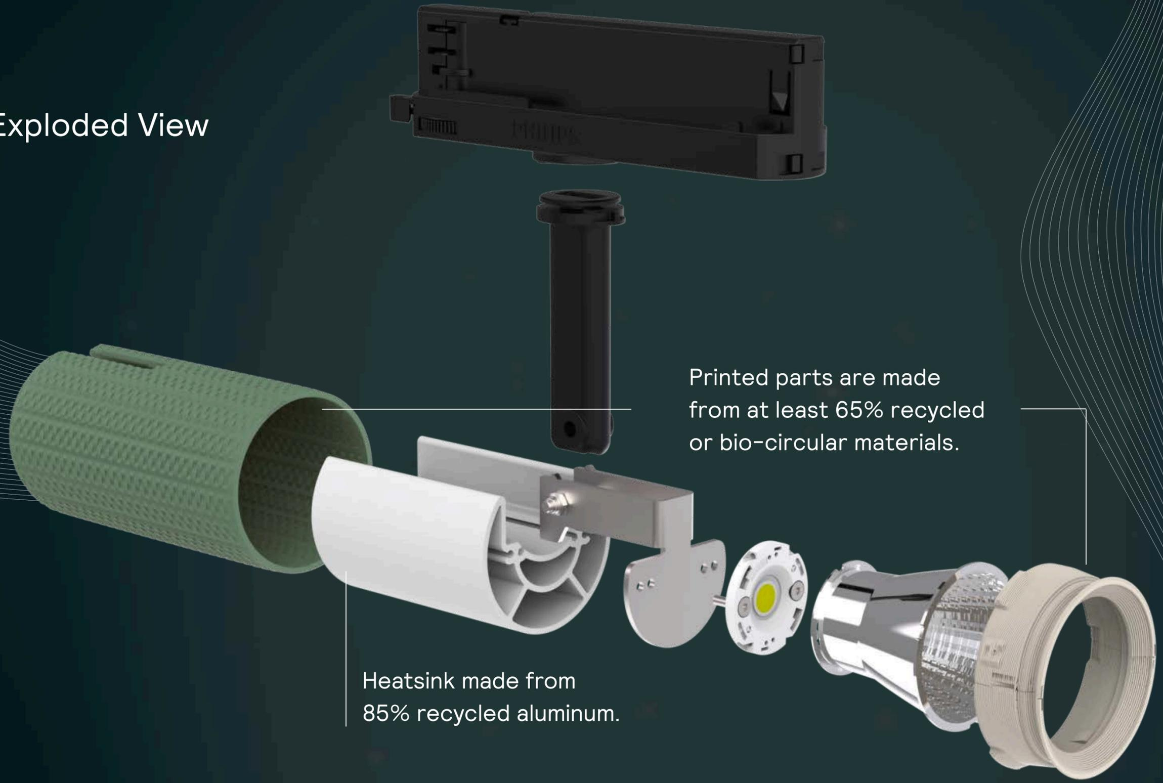
Printed parts are made from at least 65% recycled or bio-circular materials.
